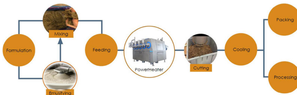
Figure 4: Basic processing flow of texturized plant protein production using POWERHEATER™ equipment.
