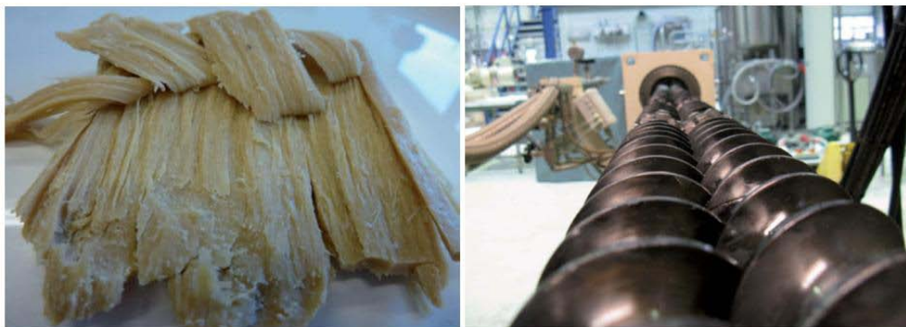
Figure 3: Example of structured protein produced by high moisture cooking extrusion and twin screw extruder with opened barrel [8].
