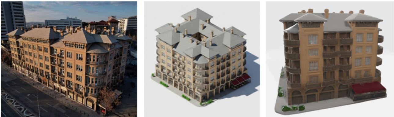
Figure 7. Three-step workflow of the proposed method illustrated using the İkinci Evkaf Apartment: (left) original building photograph, (centre) isometric daylight image generated by Gemini Flash 2.5, (right) textured 3D building model reconstructed by Hunyuan3D 2.1.
