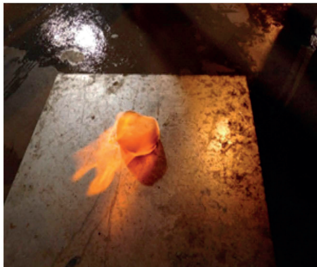
Figure 2. Images of recovered gas hydrates from the seafloor and their appearance when burned in the western Black Sea (Figure: TP-DEPARK Project Report, 2018).
