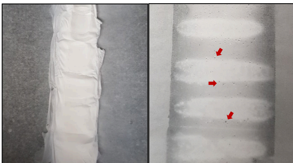
Figure 1. The smooth nanofiber layer was collected on greaseproof paper in a flat collector with PVA:water:ethanol (20:40:40, w/w/w) solution and the beaded nanofiber structure was obtained from the 20% PVA solution under high voltage and flow. (PVA: Polyvinyl alcohol; HPMC: Hydroxypropyl methylcellulose)
