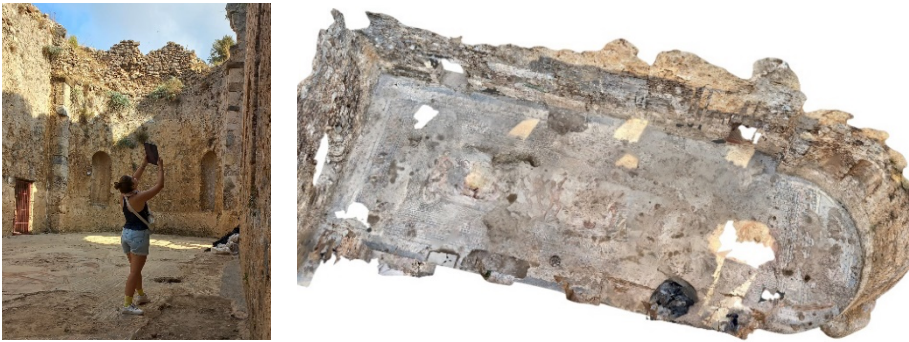
Figure 1. (left) 3D laser scanning process with the LiDAR and (right) high-quality 3D model
