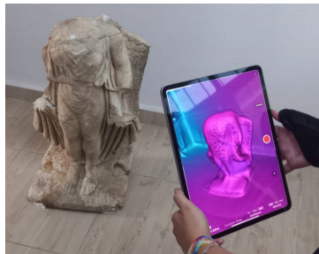
Figure 2. 3D scanning processes of a statue found in Syedra Ancient City
