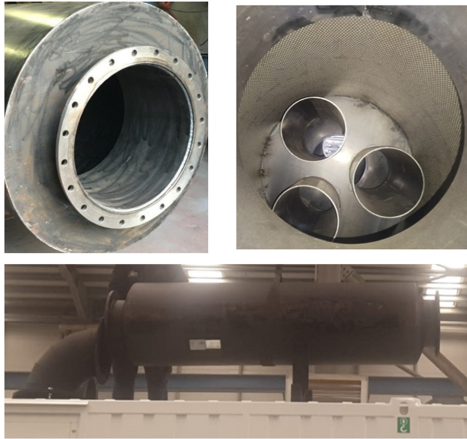
Figure 7. Silencer manufacturing stages.
